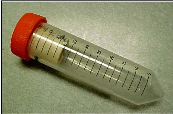
**Fig. 1.** Corning 50 ml Centrifuge Tube (Corning Incorporated, Corning, NY 14831, Item #430290)
