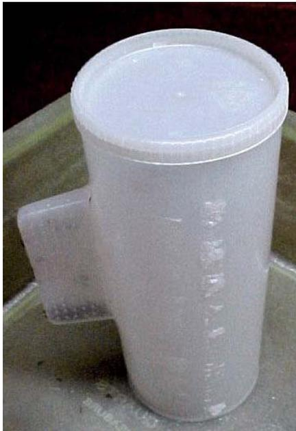
**Fig. 1.** Weep hole cover affixed to test chamber.
