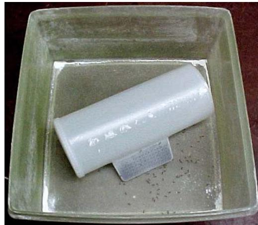
**Fig. 3.** Experimental apparatus for assessing weep hole cover effectiveness.
